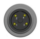
A voltage supply between pin 1 (+24V DC) and pin 3 (GND) is necessary for operation of the gripper. A jaw movement is triggered by a 24V voltage level on pin 2 or pin 4.
